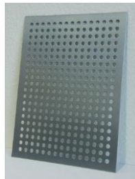
Perforation diameter 8 mm, holes in a grid spaced at 15 x 15 mm
